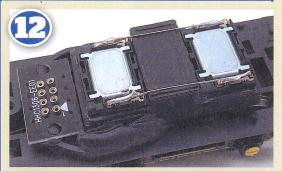
To make way for all the new components, we relocated the decoder socket to the front of the tender, just behind the front support for the tender weight. The 40mm x 22mm speaker is then fixed behind — both held in place with Black Tack — with the decoder socket wires concealed beneath the speaker.
