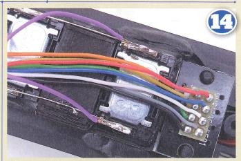
The purple speaker wires are shortened to around 50% of their supplied length and then soldered to the connections on top of the speaker.
