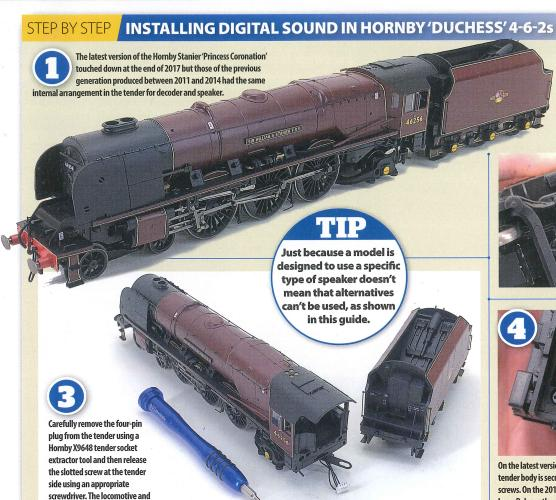
To make working on the model simpler, we find it helpful to separate the locomotive and tender. The 'Princess Coronation' models all have Homby's standard arrangement of a drawbar fixed with slotted screws at both ends and a four-wire plug to join the two halves electrically.
