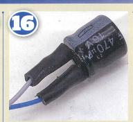
To protect the capacitor, the new soldered joints are covered with heatshrink tubing. This was put over the blue and grey wires before soldering them to the capacitor legs then shrunk with the side of a soldering iron.
