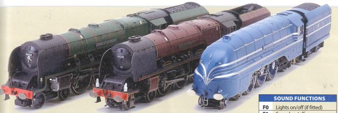
From left is the 2014 model of 46233 *Duchess of Sutherland*, the 2017 model of 46256 *Sir William A Stanier FRS* and the 2018 model of 6221 *Queen Elizabeth*, all of which have a tender mounted 8-pin decoder socket and space for a 28mm round speaker as standard. By removing the metal weight from the tender on the latest versions - not necessary on 46233 - there is ample space for a larger 40mm x 22mm speaker as shown in the step by step guide.
