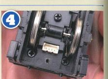
On the latest versions, both streamlined and non-streamlined, the tender body is secured to its chassis at the front by two crosshead screws. On the 2011-2014 models only a single screw is included here. Release these with a crosshead jewellers or modelling screwdriver first.
