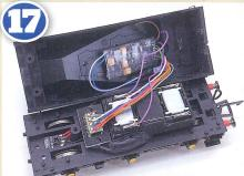
The decoder and capacitor were mounted to the roof of the tender body with Black Tack before it was refitted, taking care to ensure that none of the wires were snagged on reassembly.
