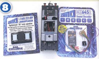
To create the ultimate 'Princess Coronation' we are going to add sound using a Zimo decoder loaded with Digitrains' Z5003A sound file, a capacitor for 'stay alive' and a Zimo LS 40mm x 22mm x 9mm twin driver 3D printed speaker.
